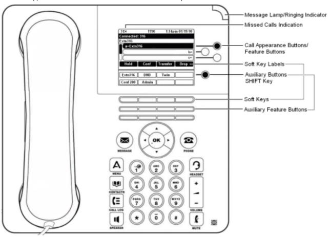
The phone supports 24 programmable call appearance/feature buttons. The labels for 3 of these are displayed in the main display and can be controlled by the adjacent buttons to the right. You can use the  $\triangle$  up/down  $\triangledown$  keys to scroll the display. You can also use the  $\blacktriangleleft$  left/right  $\triangleright$  keys to move through the button feature in pages of 3.
