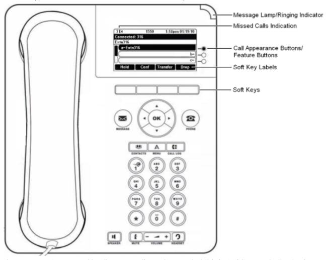
The phone supports 12 programmable call appearance/feature buttons. The labels for 3 of these are displayed in the main display and can be controlled by the adjacent buttons to the right. You can use the  $\triangle$  up/down  $\nabla$  keys to scroll the display. You can also use the  $\triangleleft$  left/right  $\triangleright$  keys to move through the button feature in pages of 3.
