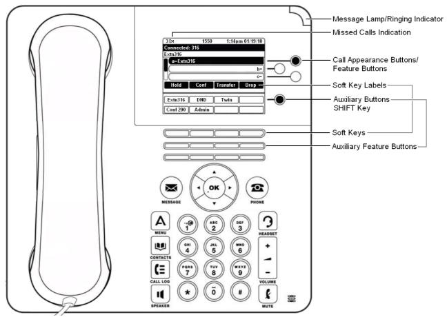
This phone supports 24 programmable call appearance/feature buttons. The labels for 3 of these buttons are visible on the main display and can be controlled by the adjacent buttons to the right. You can use the  $\blacktriangle$  up and down  $\bigtriangledown$  arrow keys to scroll the display. You can also use the  $\blacktriangleleft$  left and right  $\blacktriangleright$  arrow keys to move through the button features in pages of three.
