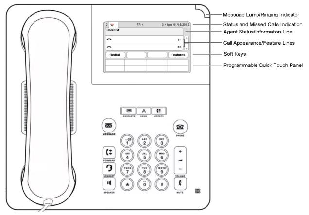
This phone supports 24 programmable call appearance/feature buttons. The labels for these are displayed in the scrollable main display along with icons for the status of the buttons.
