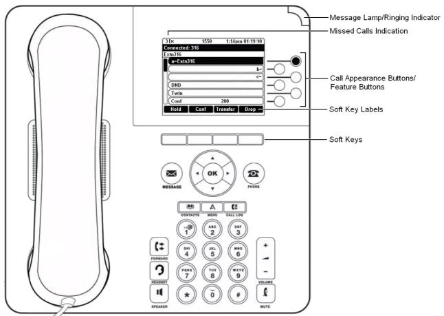
This phone supports 24 programmable call appearance/feature buttons. The labels for 6 of these buttons are visible on the main display and can be controlled by the adjacent buttons to the right. You can use the  $\blacktriangle$  up and down  $\forall$  arrow keys to scroll the display. You can also use the  $\blacktriangleleft$  left and right  $\blacktriangleright$  arrow keys to move through the button features in pages of 6.
